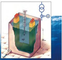
The water proof test of Busbar (with junction) meets the standard of IEC 60529 reaching IP68.
