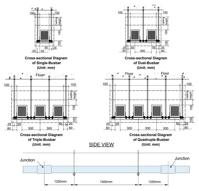
1. The installation pitch between each hanger has to comply with the standard as above. If the work condition can not meet the standard, it may be adjusted according to the condition on site. However, it must meet the requirement described in page 25 of the installation guide: minimum pitch requirement of the busbar.
